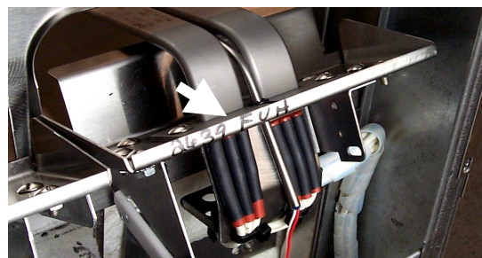
Figure 3: A shroud is provided in the retrofit kit and should be added if the raised edge (shown with the arrow) is absent from the fryer being retrofitted. A tilt-plate without the needed shroud is shown below.
